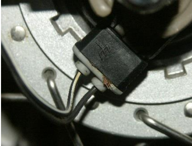
1) Look for connector at wheel hub
