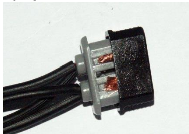
5) Strip isolation for all wires by 20-25mm
