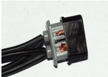
5) Strip isolation for all wires by 20-25mm
